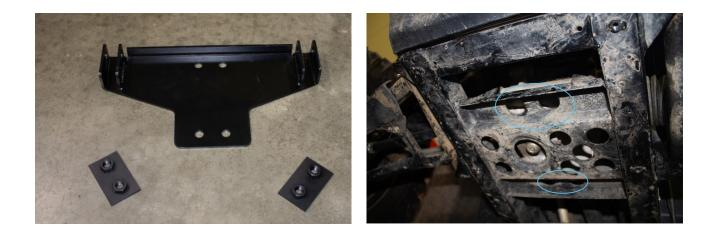
3. Hold mount to frame and insert provided bolts to threaded brackets using a washer and lock washer on each bolt.
